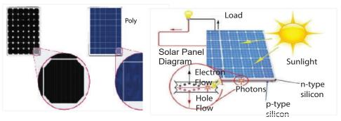
Figure 6: Photovoltaic Polycrystalline and Mono-crystalline Solar Panels
